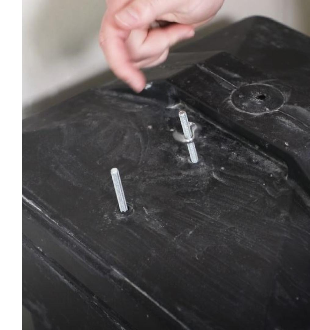
Drill a larger hole on the opposite side of the lid to make an opening for the power cable to run through.
