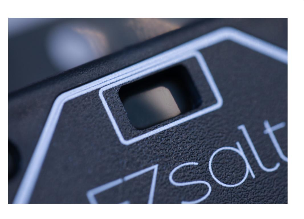
The EZsalt Sensor uses a laser ranging sensor to measure the distance between itself and the salt.
